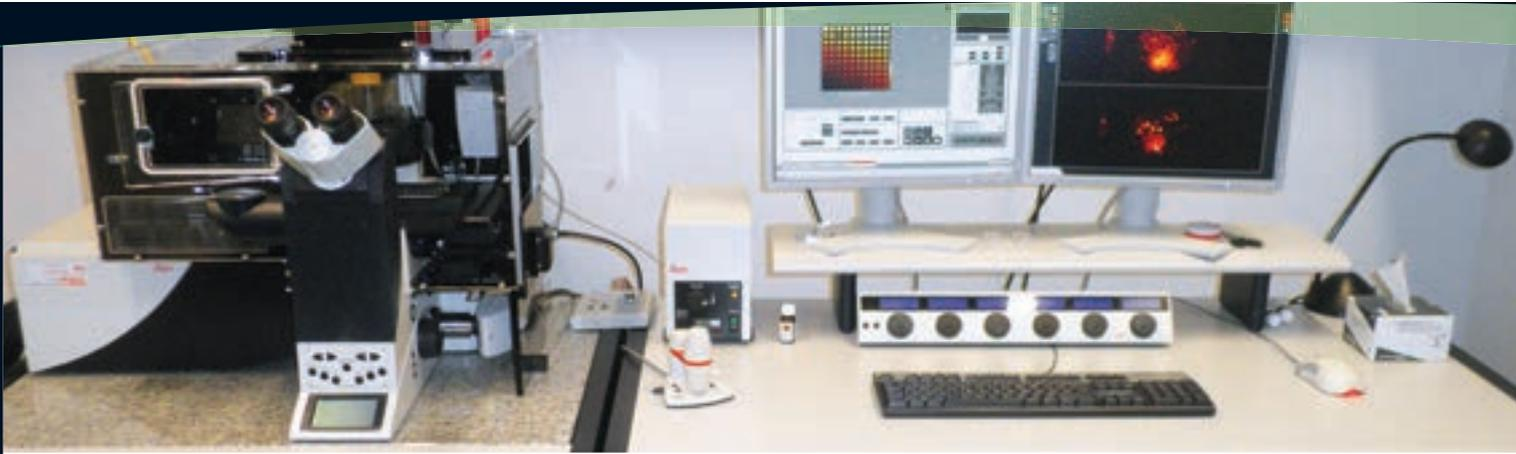
Figure 2: Leica TCS SP5 automatic confocal microscope with incubation chamber for live-cell imaging (Photo: Nina Beil).
