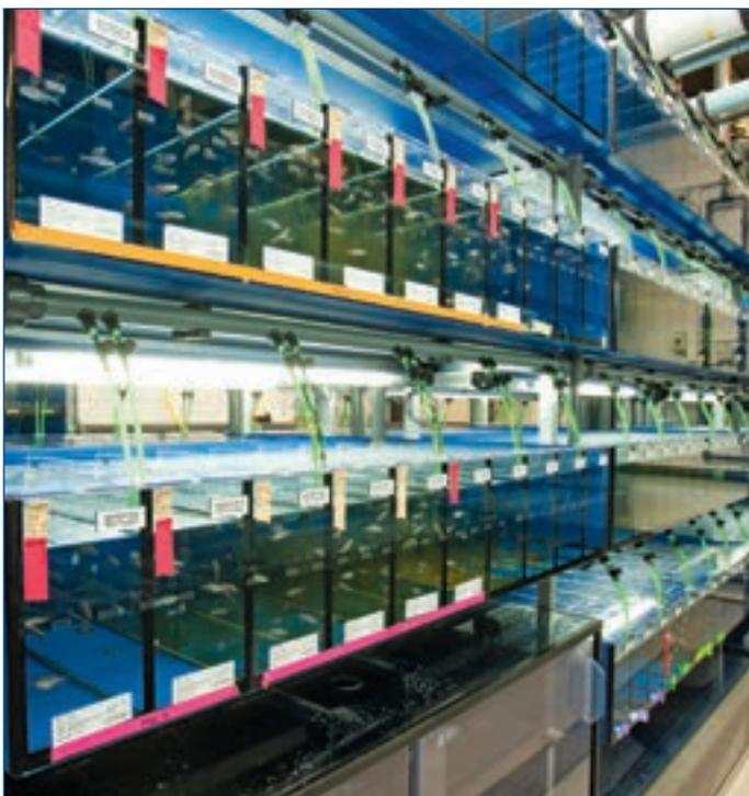
To provide healthy conditions for the animals, aquaria are continuously supplied with freshwater and all important parameters, such as pH, temperature and water supply, are electronically monitored.
